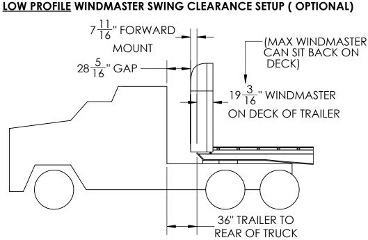
NOTE: WINDMASTER CAN FIT ANYWHERE BETWEEN STANDARAD AND LOW PROFILE SETUP
