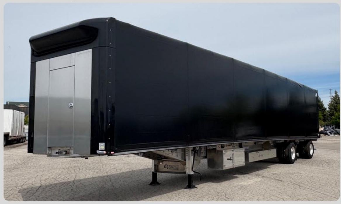
Windmaster GR8LOOK is a Sleek Integrated Aerodynamic 3 Pcs Modular Front Bulkhead. CFD Tested, results in comparison to a 100" high alum. flat bulkheads at 65 MPH proved Reduce Wind Drag by 5.89 % and enhance fuel savings 2.95%.
