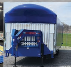
Hydraulic Tilt Deck GN w/ LCS Round Top Windmaster Aerodynamic SLIDEKIT System. Comes STD 66" Side Ht. / 90" Center Ht. Available 96" Side Ht. / 120" Center Ht.
