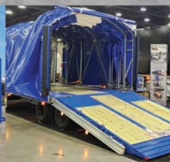
Hydraulic Tilt Deck GN w/ LCS Round Top Windmaster Aerodynamic SLIDEKIT System. Comes STD 66" Side Ht. / 90" Center Ht. Available 96" Side Ht. / 120" Center Ht.
