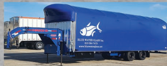
Hydraulic Tilt Deck GN w/ LCS Round Top Windmaster Aerodynamic SLIDEKIT System. Comes STD 66" Side Ht. / 90" Center Ht. Available 96" Side Ht. / 120" Center Ht.
